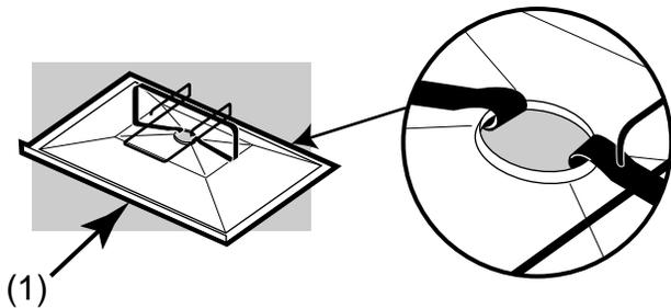
Slide the bottom tray onto the mounting rails under the cooking box with finger grip toward you(1).
