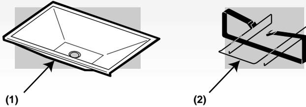
Hook the ends of the catch pan holder into the hole in the slide out bottom tray. **The front of the catch pan holder must be on the same side as the finger grip(1) of the bottom tray.**
