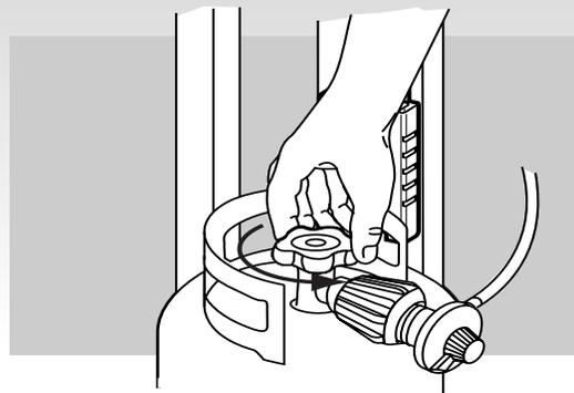
If there is a leak, turn off the gas and tighten the fitting. Turn the gas back on and recheck with the soap and water solution.
