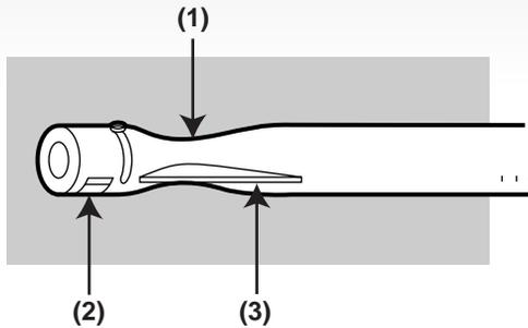
The Weber Spider Stopper™ Guard(1) is factory installed. It fits tightly around the air shutter section of the burner tube and the valve, thereby preventing spiders and other insects access to the burner tubes through the air shutter openings.
